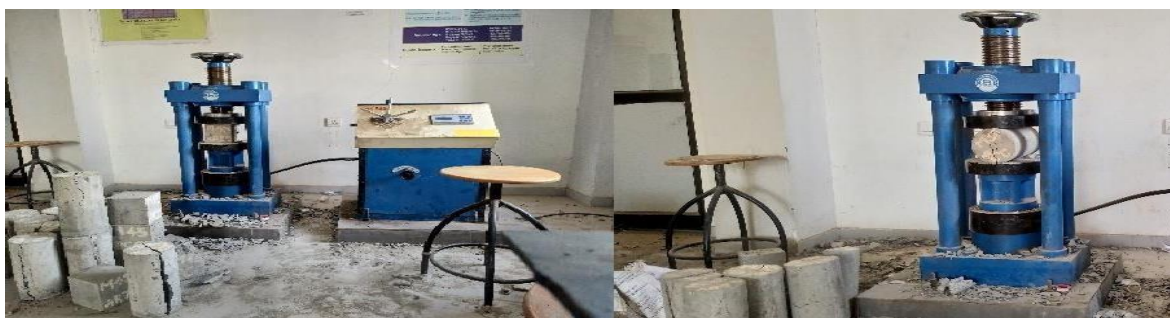
Fig. 3 Split Tensile Strength test
