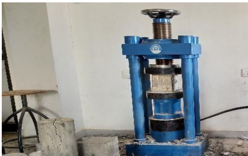
Fig. 2 Compressive Strength test
